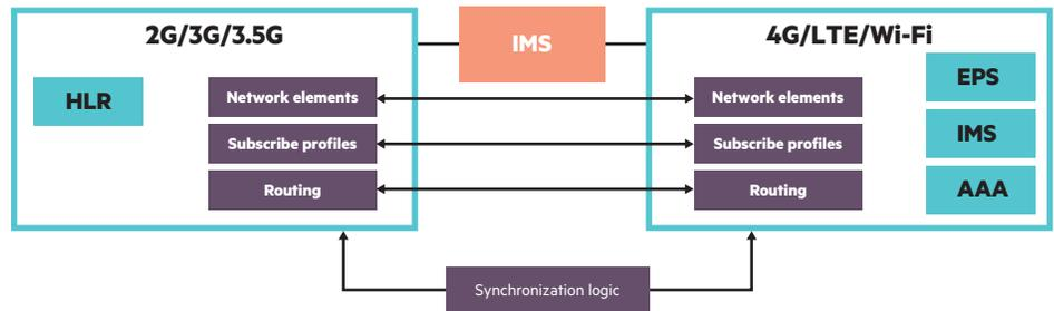
**Figure 2:** Maintain and bolt-on convergence design
