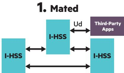
Figure 11: Mated servers. Mated Triple shown
