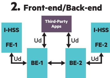
Figure 12: Front-End/Back-End. Mated pair of FEs/BEs shown
