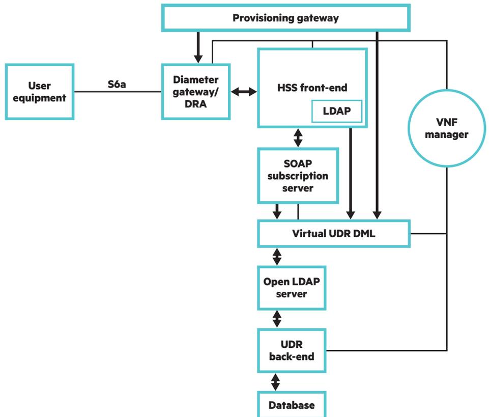
Figure 2: Open design SDM reference architecture
