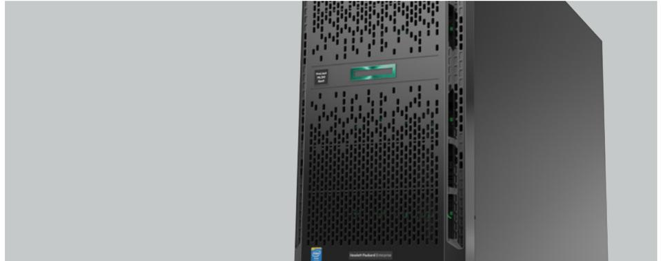
Their HPE ProLiant ML350 Gen9 server has dual power supplies and other redundancy features, which are very important to the firm. Plus, it comes standard with the latest Intel Xeon processors, HPE DDR4 SmartMemory, and support for up to 48 small form factor (SFF) drives. The firm uses 10K RPM SAS drives, configured in a RAID 5 array.
