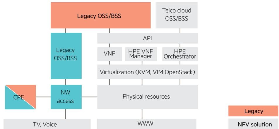
**Figure 2.** Deployed architecture
