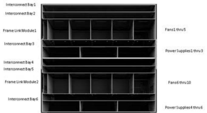
HPE Synergy 12000 Frame - Rear View
