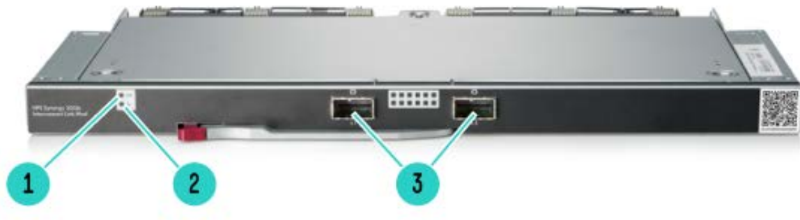
Figure 1 HPE Synergy 20G Interconnect Link Module Bezel
