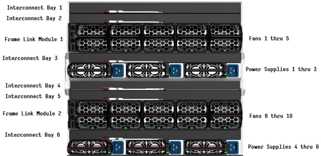
HPE Synergy 12000 Frame - Rear View
