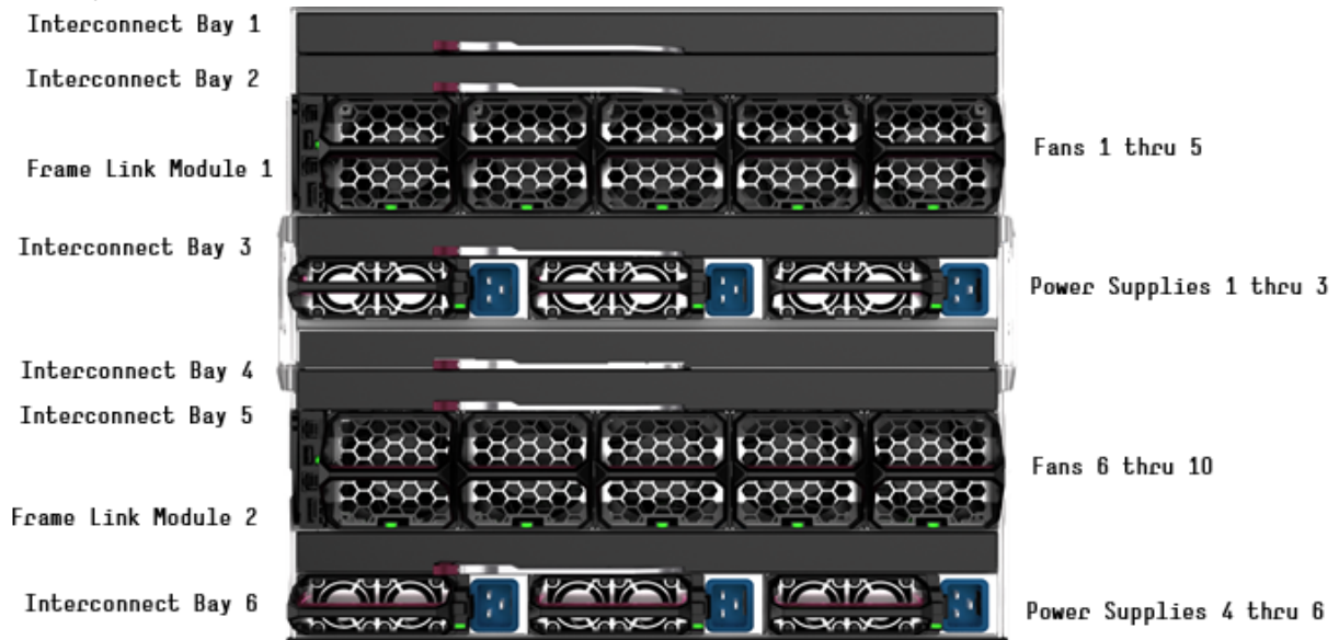
HPE Synergy 12000 Frame - Rear View
