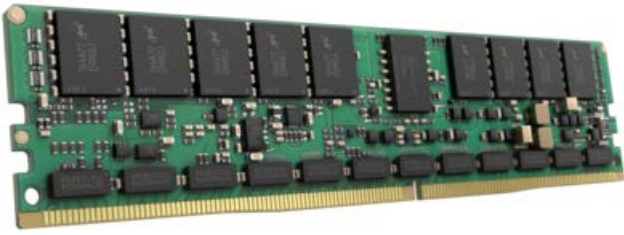
Figure 1. HPE 8GB NVDIMM module
