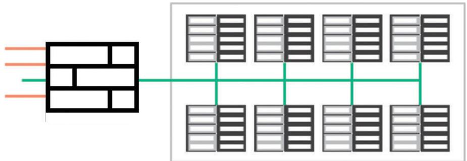
**Figure 2.** Traditional datacenter security policies focused on perimeter firewalls, but had few controls within the datacenter for east-west traffic.
