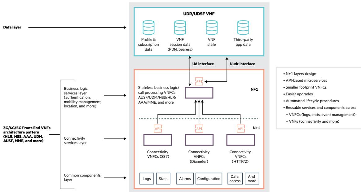
Figure 1. Telco Cloud data layer conceptual view
