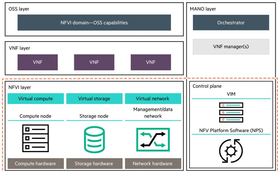
Figure 2. HPE Telco Blueprint Architecture
