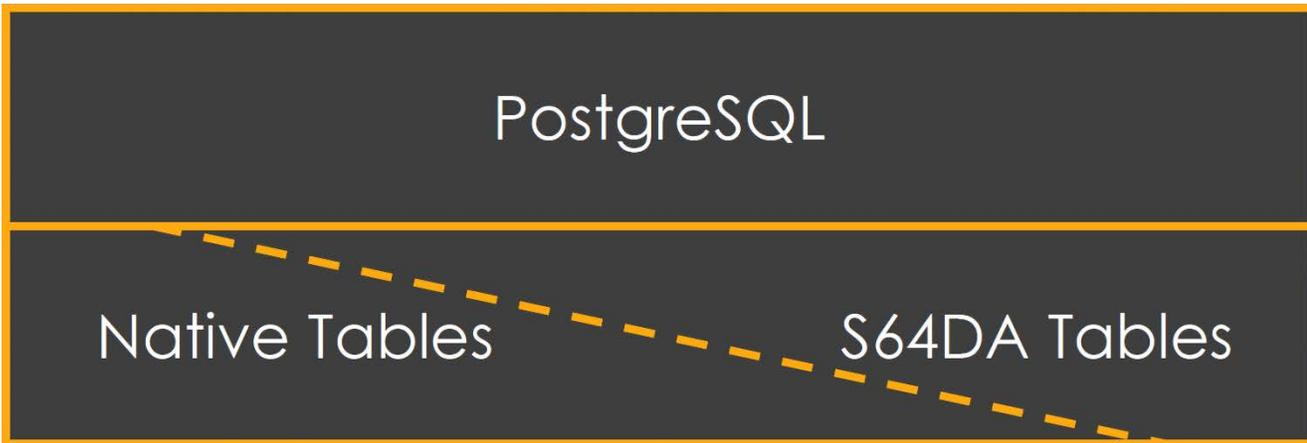
**Figure 1.** Intel Arria 10 GX FPGA with Swarm64 DA supports all of the database's functionality via the PostgreSQL native table format or a large sub-set via the Intel Arria 10 GX FPGA with Swarm64 DA tables, created as "Foreign Tables".
