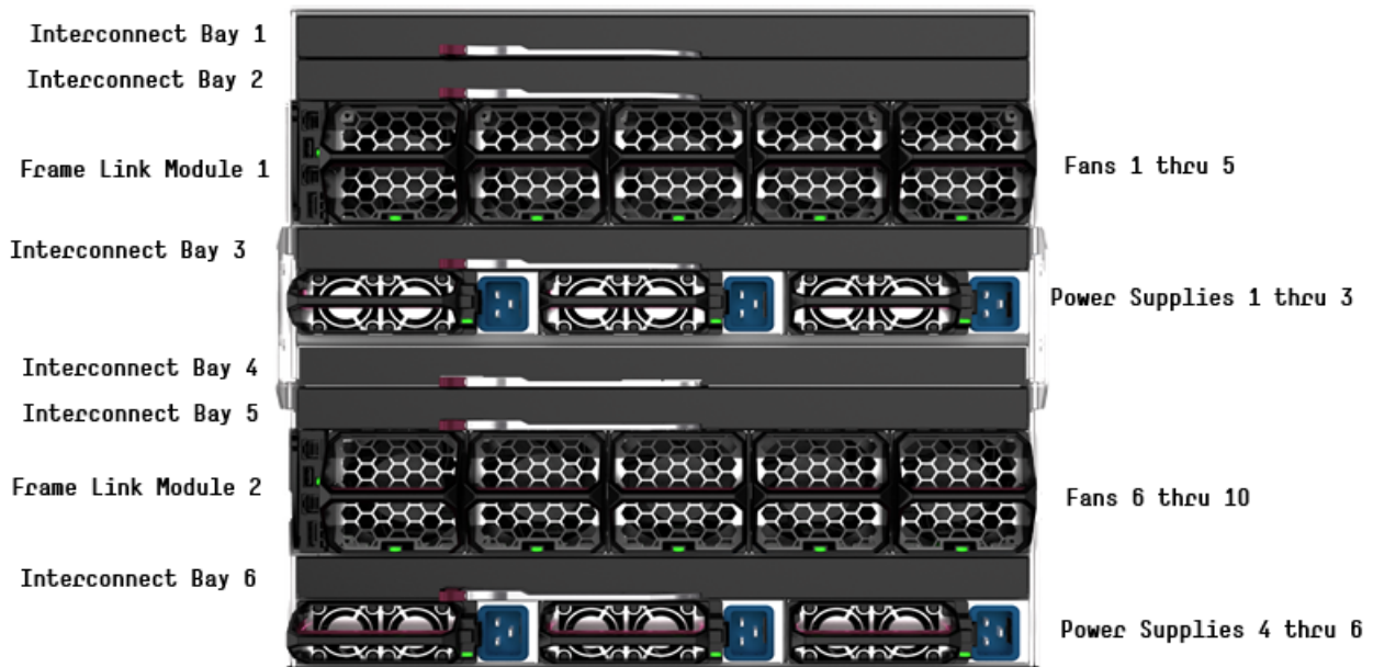
HPE Synergy 12000 Frame - Rear View
